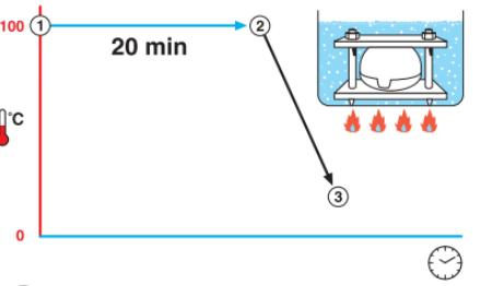
**GB** ① Start curing process in hot water + Maintain water temperature ② Stop curing + Air cooling to ambient temperature ③ End of total curing process
